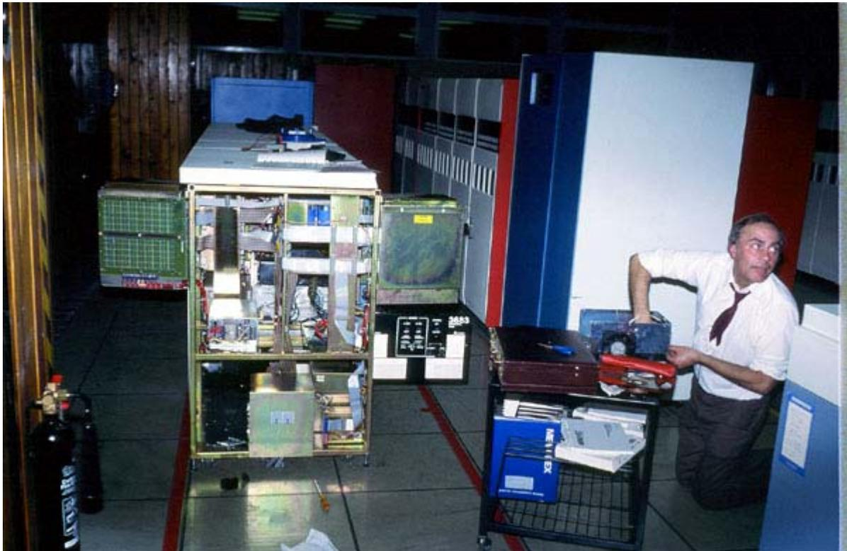
This is a photograph of a Memorex 3680 disk drive unit being repaired, as was too often the case. At the bottom is a power supply and out of sight, a large electric motor that turned the pack of disks via a belt. Above is control circuitry, and just visible a bit of the disk storage FRU itself.
